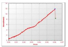
Figure.13. Stress strain graph of NaOH and HCL treated composite
